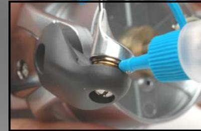
Lightly oil line roller assembly using Shimano® Bantam™ Oil. Regular oiling (after every fishing trip or two) will greatly increase the life expectancy of the line roller bearing.
