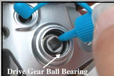
Drive Gear Ball Bearing
