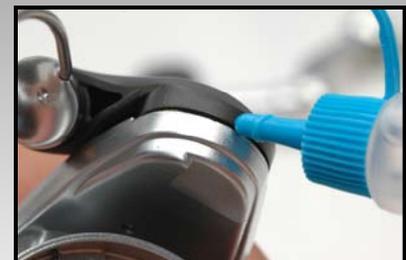
Oil bail arm assembly to maintain smooth and consistent bail operation. For further assistance, or to order parts, contact **Shimano® Customer Service** at **1-877-577-0600**.
