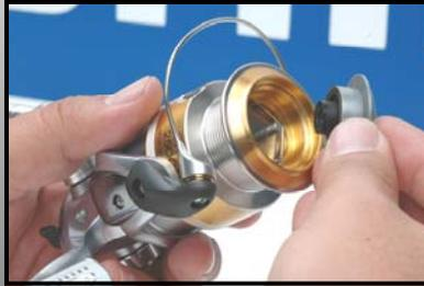
Remove spool assembly by turning drag knob counter clockwise. On Reels equipped with a rear drag, spool assemblies are release via push button. and handle assembly.
