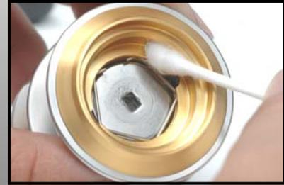
Inspect spool assembly for damage. Pay special attention to the spool lip, as damaged or chipped spool lips will consequently cause premature wear on fishing line.
