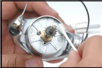
Clean exterior of reel with cotton swabs and isopropyl rubbing alcohol. Clean off excess oil, grease, salt deposits or debris. Keeping reels clean helps prevent costly
