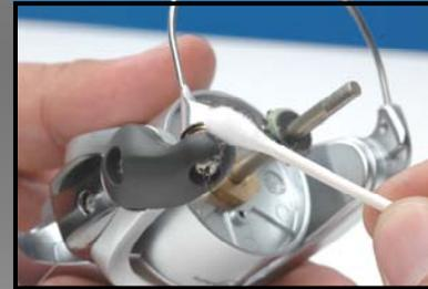
Inspect and clean line roller assembly. Use a cotton swab to “feel” if the line roller bearing or bushing needs to be replaced. A rusted or worn bearing will be most noticeable during line retrieval.
