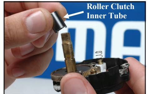
The roller clutch inner tube should be installed with the prongs facing down toward the metal drag plate. Use a cotton swab to apply a very light coat of Bantam® Oil on the outside of the inner tube and to the inside of the roller bearing.
