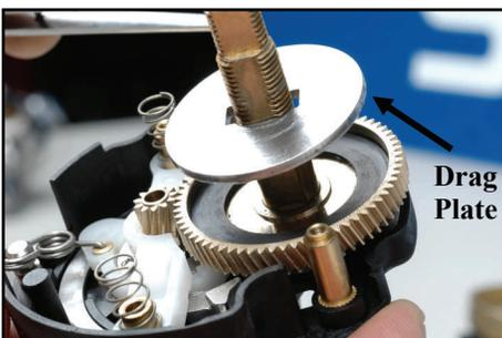
Remove the metal drag plate to expose the drag washer. On older Calcutta® models, the drag washers are made of a fabric material. The Calcutta®B drags are Dartanium (carbon like material). Dartanium drags are very fragile, so take extra caution not to break them! Clean inside of drive gear and drag plate with cotton swabs and alcohol.
