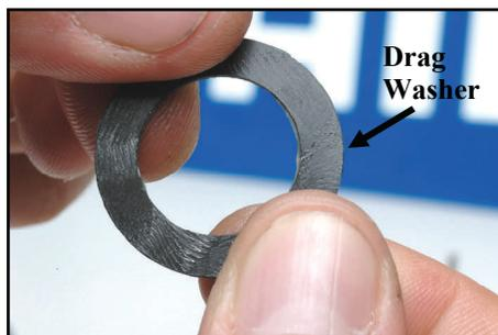
Grease Dartanium drags with a light coat of Shimano® Drag Grease. The old style fabric drags will require more grease than Dartanium drags. More grease= smoother drag. Less grease= more drag pressure. Excessive grease will yield insufficient drag pressure.
