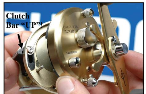
**Important:** When re-installing the sideplate, make sure that the clutch bar is held in the “up” position, otherwise, the clutch won’t work. Run the **Diagnostic Procedures** again to ensure proper function of the anti-reverse and/or drag.
