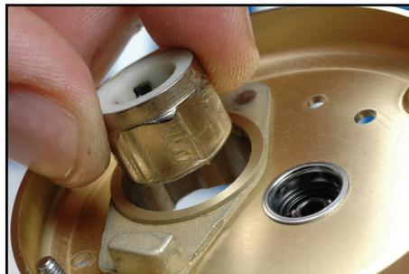
With the old roller clutch bearing out, clean off any debris, rust or excess grease. The new bearing is now ready to be installed as shown above.
