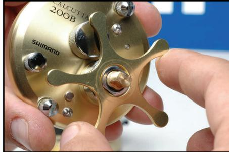
Use a small screwdriver to remove handle nut plate, handle nut and side plate screws. Back-off star drag and remove washers underneath.
