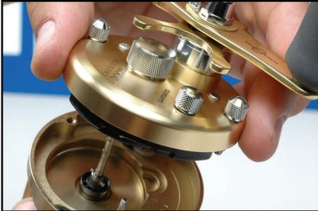
Loosen thumb screws and remove side plate. **Note:** When closing, never over torque thumbscrews with a screwdriver, as they will break.
