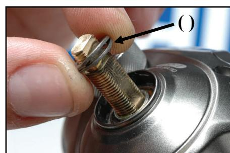
**Important:** After re-installing the sideplate, re-install the drag star springs as depicted above- ( ). If they are not installed correctly, the drag range will be affected. Run the **Diagnostic Procedures** again to ensure proper function of the anti-reverse and/or drag.
