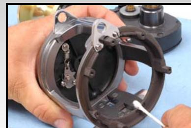
Clean Frame with isopropyl rubbing alcohol using a toothbrush and/or cotton swabs.
