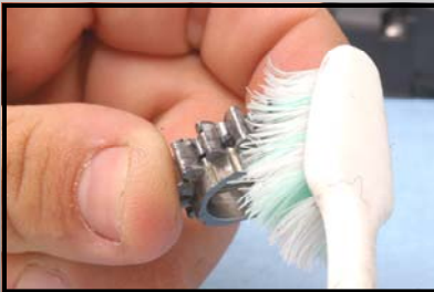
Clean Pinion Gear (s) and apply a light coat of grease.
