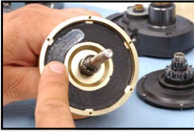
With the Cooling Shield removed, clean and lightly apply Shimano® Drag Grease to the Drag Washer.
