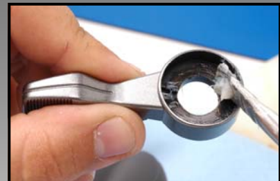
Grease Drag Control Lever with Shimano® Drag Grease.
