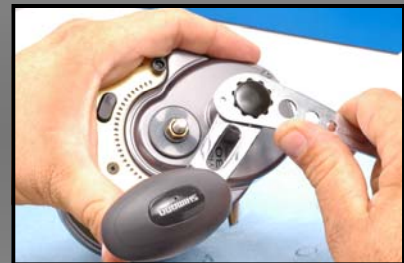
For Single Speed Reels , Remove Handle Bolt Screw and Handle Screw with supplied wrench.
