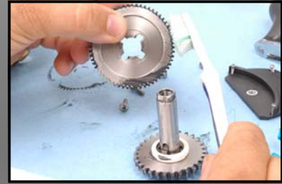
Clean Drive Gear (s) and Drive Shaft and lightly re-grease.
