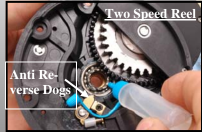
Grease Bearing and oil Anti-Reverse dogs - ( Two Speed Reel )
