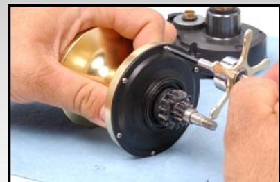
Remove Cooling Shield Screws, Pinion Gear (s) and subsequently 1 remove the Cooling Shield along with the Drag Plate.
