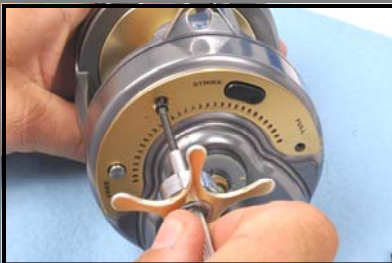
Remove Lever Quadrant Screws and Lever Quadrant.
