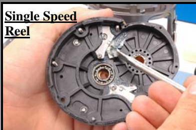
On Single Speed Reels , lightly grease Anti-Reverse Dogs.
