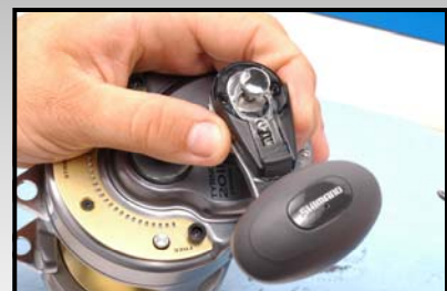
For Two Speed Reels , reinstall the Handle Bolt, Handle Bolt Plate, Slide Plate and Slide Plate Spring, followed by the Screw and Push Button Shield and Screws. Lastly, 2 check if the reel is shifting properly.
