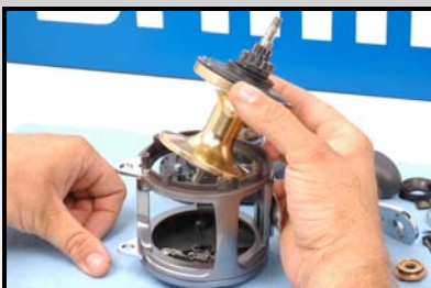
Extract spool Assembly from Frame.
