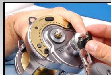
Reinstall Handle Assembly with supplied Shimano® wrench for Single Speed Reels , or crescent wrench for Two Speed Reels .
