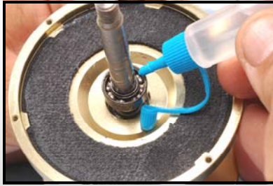
Check Spool Bearings for rust or wear. Apply only 1 drop on each bearing, as excessive oil will adversely affect drag performance.
