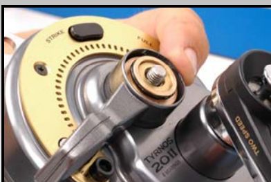
With the Drag Control Lever in the freespool position, install the Lever Thrust Body. Important: Make sure that it is properly seated all the way down, or else Drag Control Lever will not move properly.
