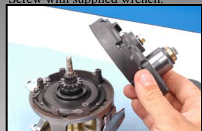
Remove Side Plate Screws and remove Right Side Plate.
