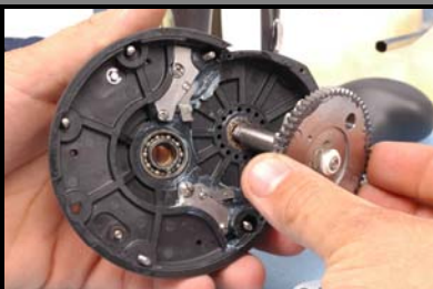
Reinstall Drive gear.
