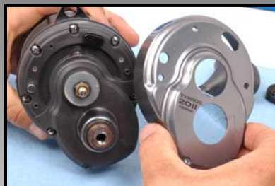
Remove remaining Side Plate Screws and remove Right Side Plate Cover.
