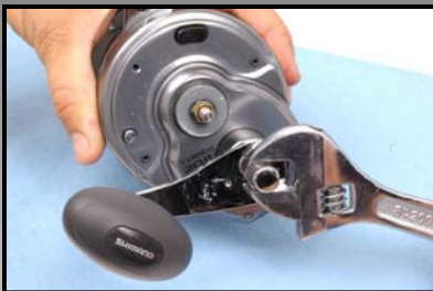
Remove Handle Bolt from Two Speed Reel with a crescent wrench.
