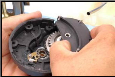
Remove Right Side Seal and Screws to access Drive Gear (s).
