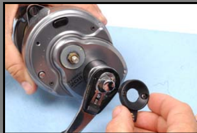
For Two Speed Reels , remove Push Button Shield and Slide Plate.
