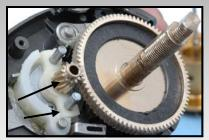
Reinstall drive gear, drag washers, yoke and pinion. Take care not to damage gear threads. Note the proper orientation of yoke and pinion gear.
