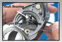
Lightly oil Super Free<sup>TM</sup> support bearing and drive shaft bearing.
