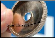
Clean drive gear and apply Shimano® Drag Grease on the threads of the gear.
