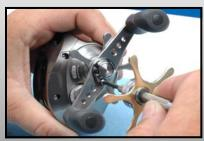
Use a small Phillips or flathead screwdriver to remove handle assembly.
