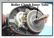
Reinstall yoke springs and roller clutch inner tube. Reinstall right side plate and side plate screws.
