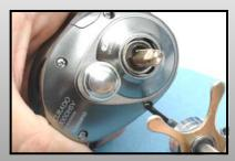
Remove side plate screws. It is always a good idea to lay out the parts in order to aid in reassembly.
