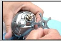
Use a 10MM nutdriver or wrench to remove handle nut. Thereafter, remove star drag, spring, and washers
