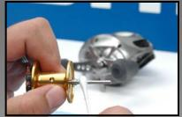
Inspect and clean spool assembly. Clean spool shaft and oil spool bearing or bushing if applicable. **Note:** Do not grease spool shaft, as it will affect freespool adversely.
