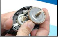
Remove drive gear, drag washers, pinion gear, yoke, yoke springs.
