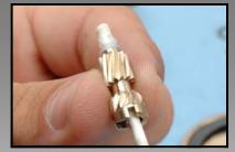
Clean the inside of the pinion gear for optimal freespool performance.
