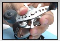
Reinstall star drag, washer, handle assembly. Tighten handle nut with 10MM nutdriver or wrench.
