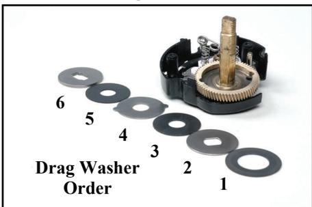
Note the above photo for the order of the drag washers. The Dartanium® washer with the large diameter hole(1) goes first into the drive gear. Subsequently followed by the thin keyed washer(2), drag washer(3), eared washer(4), drag washer (5), and lastly the thick keyed washer(6).
