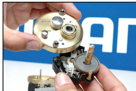
The sideplate is now ready for removal. Be careful not to drop or lose the yoke springs as they are hard to find!
