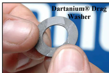
Apply a light coat of Shimano® Drag Grease to Dartanium® drag washers. More grease= smoother drag. Less grease= more drag pressure. Excessive grease will yield insufficient drag. **Dartanium® drags are fragile.** Take care not to break them!
