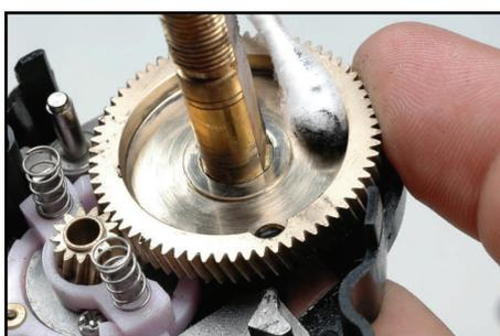
Clean drag residue, grease or oil from metal washers and drive gear with cotton swabs and rubbing alcohol. Most of the time, the drag washers are still usable after cleaning and servicing.
