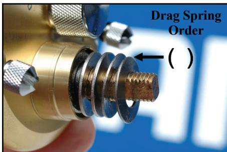
Note the proper order of the star drag spring washers above. Improper ordering will affect drag range and overall drag performance. **(thick thick) (thin thin).** These four washers are followed by the flat star drag spacer.
