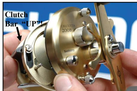
**Important:** When re-installing the sideplate on Calcutta® sizes CT50-CT400, make sure that the clutch bar is held in the “up” position, otherwise, the clutch won’t work. Run the **Diagnostic Procedure** again to ensure proper function of the drag.
