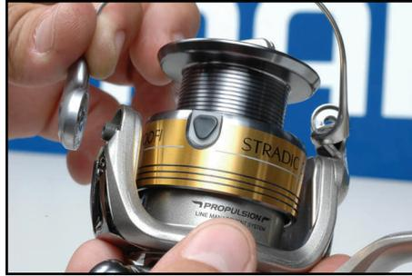
If replacing the bail wire, remove opposite screw as well. It is not necessary to remove this screw if only a line roller bearing replacement is being performed.
