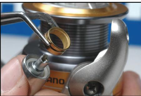
Reassemble line roller components onto bail wire assembly. Add Shimano® Bantam® Oil to the line roller bearing to help keep it properly lubricated. Oiling after use, especially in saltwater is a good way to maintain the line roller assembly.
