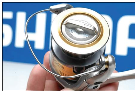
Replacement of line roller bearing and/or bail assembly is now complete.
