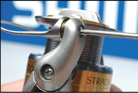
Using a small screwdriver, remove the above depicted screw. These bail assembly screws typically have thread sealant on them, so be careful not to strip them.
