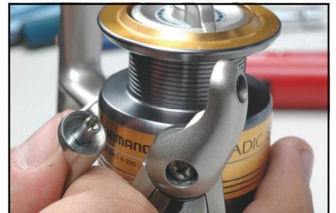
If changing the bail assembly, attach the new bail first with screw opposite of the line roller assembly first.
