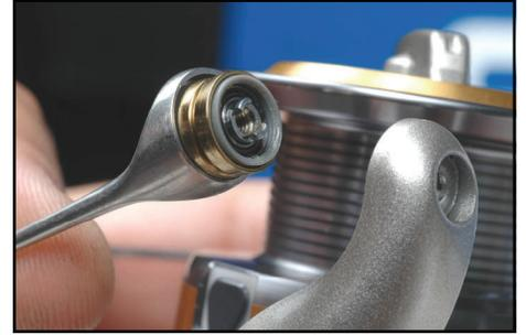
Pay close attention as to the order of the internal parts of the line roller assembly. The order of the components vary from model to model. Refer to schematics.
