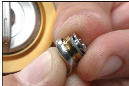
If changing the bail wire, reassemble the components of the line roller.
